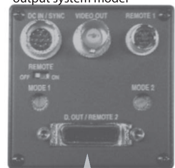
Conventional MDR-26 CameraLink Connector [39.7 x 12.9 mm]
