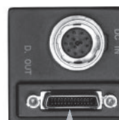
Small SDR (Mini-CameraLink) Connector [24.4 x 9.0 mm]
